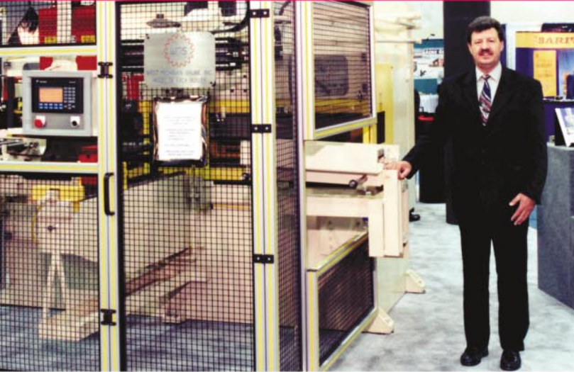
West Michigan Spline President Gary Hill at the 2001 AGMA show with a Model 36 spline rolling machine with auto-load capacity.
